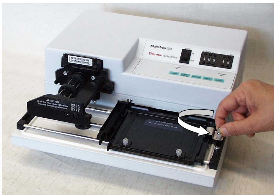
Fig. 6.12 Loosening the screws on the right of the plate carrier
