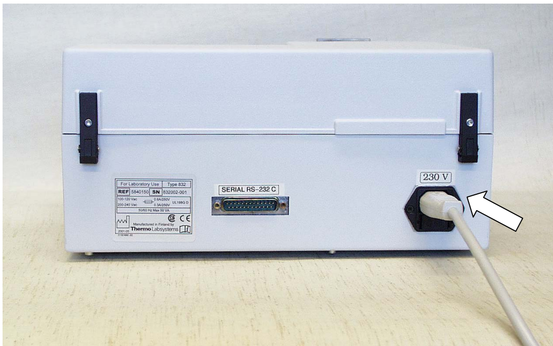
Fig. 5.3 Connecting the mains supply cable
