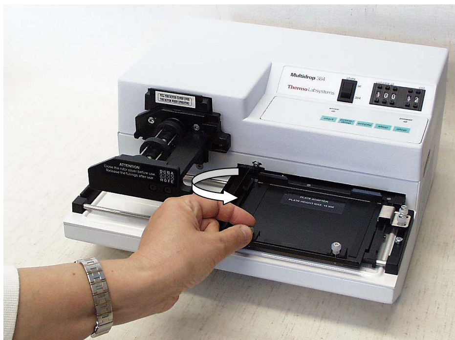
Fig. 6.13 Loosening the screws at the front of the plate adapter
